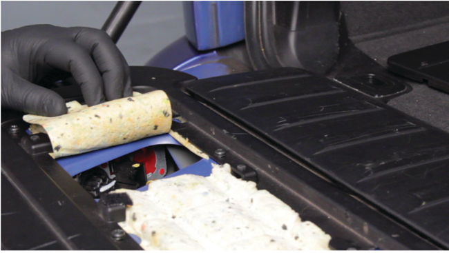
17) Disconnect the inner tail light harness.
