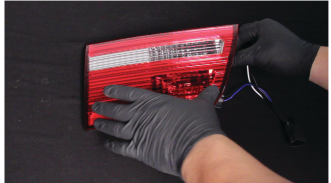
20) Transfer the reverse lamp bulb to the white and black wire socket of the Spyder inner tail light. Never touch exposed bulbs with bare hands. (EU models only: Transfer the reverse lamp bulb to the blue and black wire socket)
