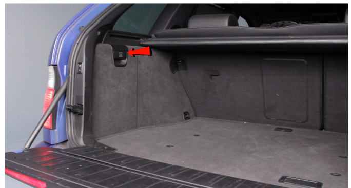
2) Open the tailgate access panel.
