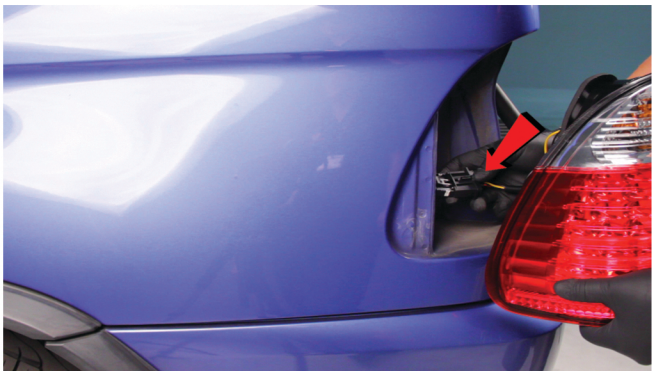
7) Connect the Spyder tail light wiring harness to the OEM tail light. Then disconnect the red and green harness clip and remove the turn signal socket from the Spyder tail light.
