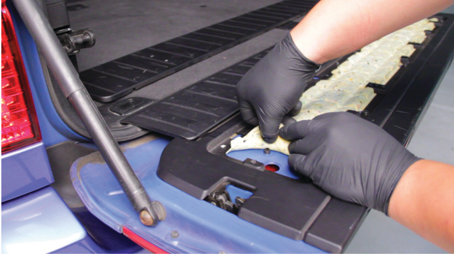
23) Reinstall the 8mm bolt hidden underneath the sound deadening.
