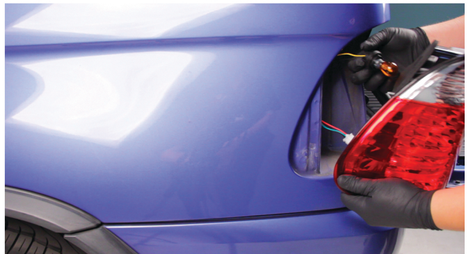
10) Reinstall the turn signal bulb into the Spyder tail light.
