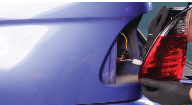
9) Reconnect the red and green harness clip to the Spyder tail light.
