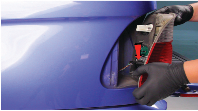
5) Disconnect the outer tail light wiring harness.
