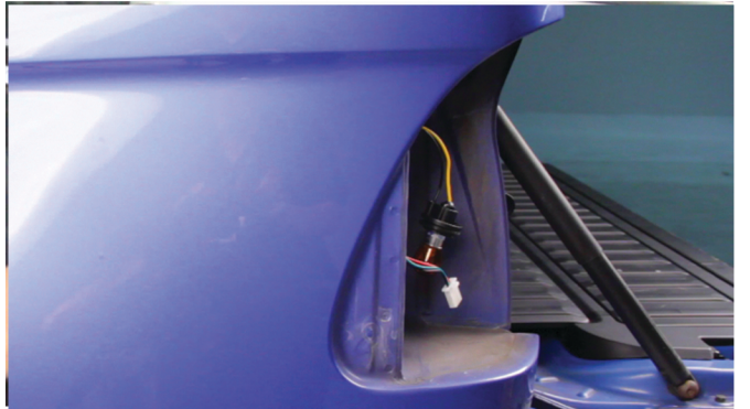
8) Feed the turn signal socket through the opening in the body as shown to avoid pinching the harness when you seat the tail light.
