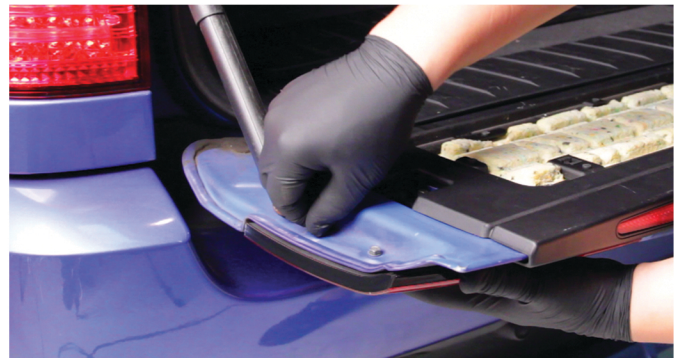
22) Reinstall the [2x] 8mm bolts securing the inner tail light along the edge of the tailgate.
