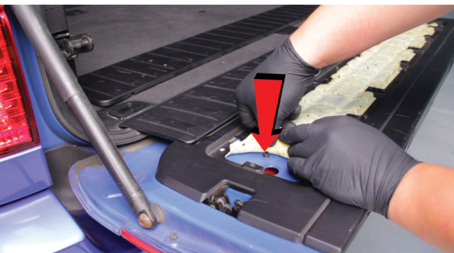
15) Peel back the sound deadening to expose and remove the 8mm bolt hidden beneath it.
