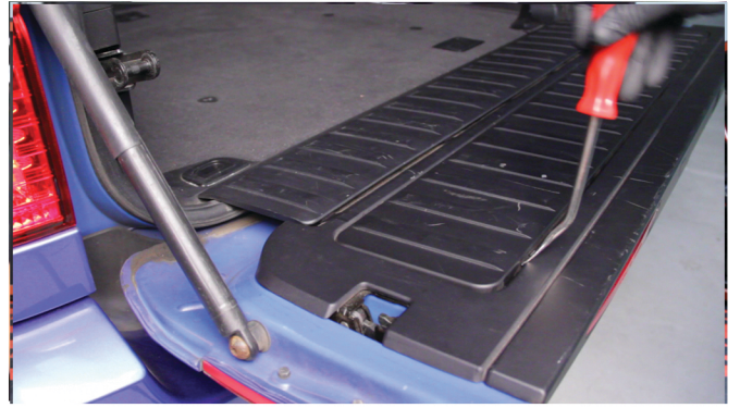
14) Moving on to the inner tails, use a panel popper or flathead to pop the tailgate cover panel free. The panel pops up from the rear and opens forward.
